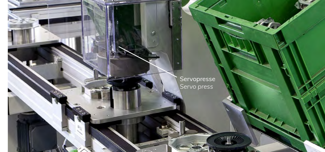
Passive Bandabsenkung | Passive belt movement
